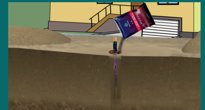
Step 4. With rod inserted, fill the hole with Advance Ground Enhancing Compound
