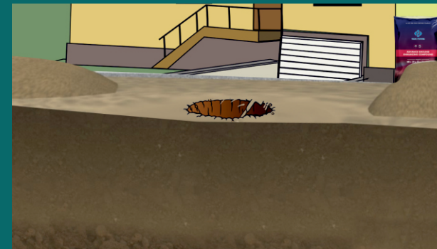
Step 1. Dig a hole with Auger
