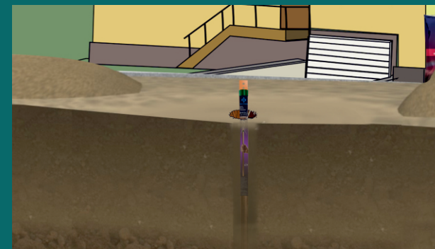
Step 3. Insert the TruePower Earthing rod
