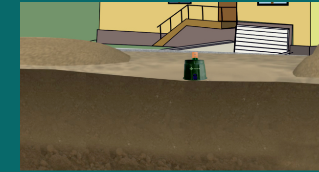
Step 6. Place the TruePower Earthpit Cover
